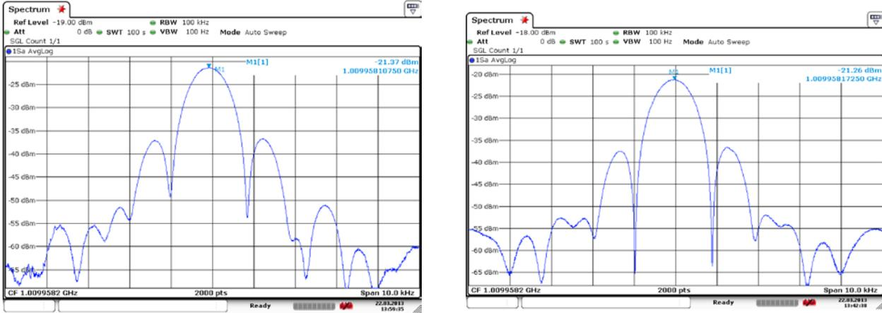
Figure 10: Left: Elevation pattern taken from the Schöckl mountain, 4.06°...6.06°, rate=0.02°/s ; Right: Azimuth pattern taken from the Schöckl mountain, 3.75° ... 5.75°, rate=0.02°/s
