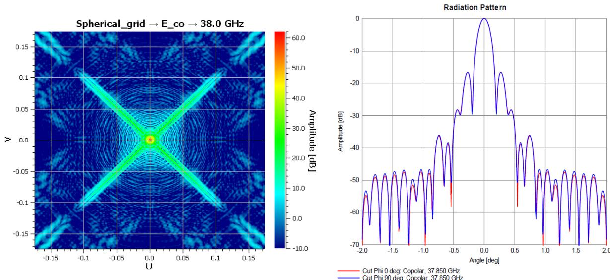
Figure 4: 3D Radiation pattern with struts influence @38GHz and right the RX antenna pattern.
