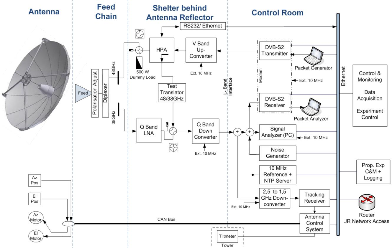
Figure 1: Architectural Design of the Q/V band GS Graz
