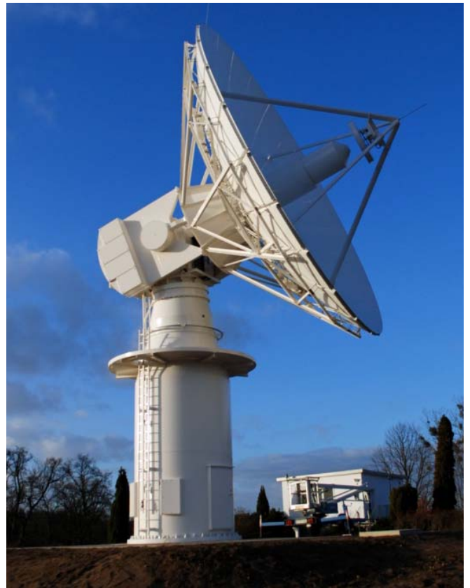
Figure 6. 11.5 m S-/X-/K-Band Antenna System installed and ready for operation
